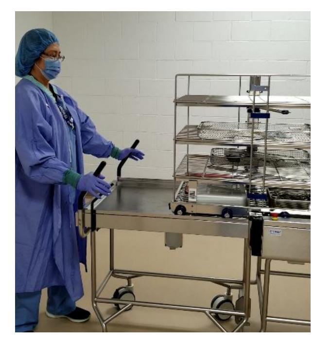
Automatic loading and unloading on washer-disinfectors and sterilizers reduces pushing and pulling needs of staff. Locking wheels and sensors add two levels of security for each conveyor. Emergency stops on each automated component results in improved ergonomics.
