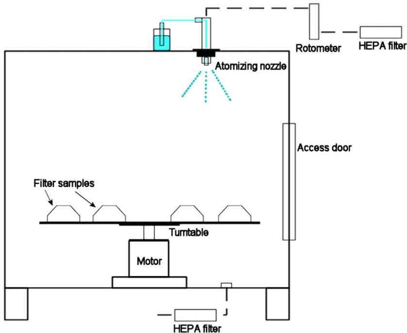
Fig. 1. Schematic of the aerosol test system.
