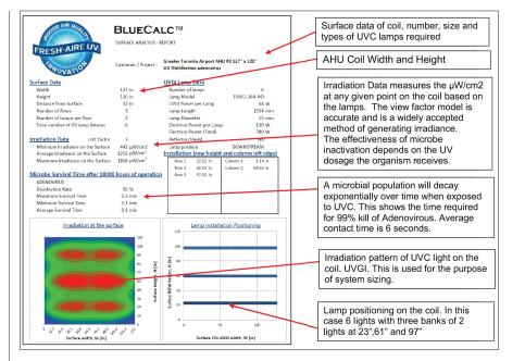
The radiant energy, or dosage, delivered to a coil surface is dependent on UV intensity, the duration of exposure, and the lamp to coil distance.
