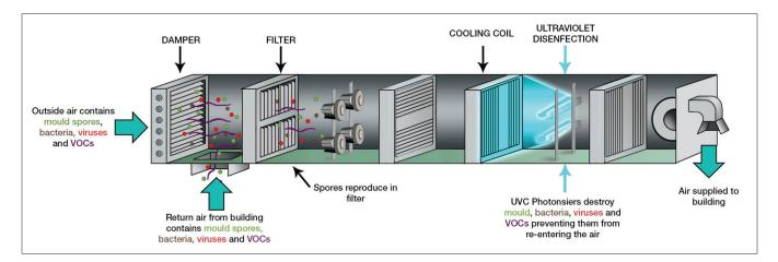
clean, biofilm-free coils, improving equipment efficiency.
